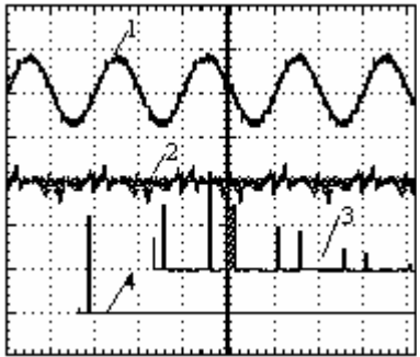
Fig. 8. Experimental results ((1). Grid current 20A/div; (2) Output current of APF 20A/div; (3). Spectrum of output current of APF 5A/div; (4). Grid current spectrum 5A/div. 10ms/div)
