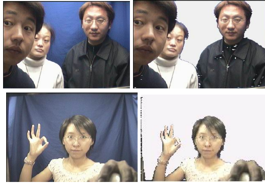
Fig. 4. The segmentation effect of threshold obtaining based on histogram peaks distribution
